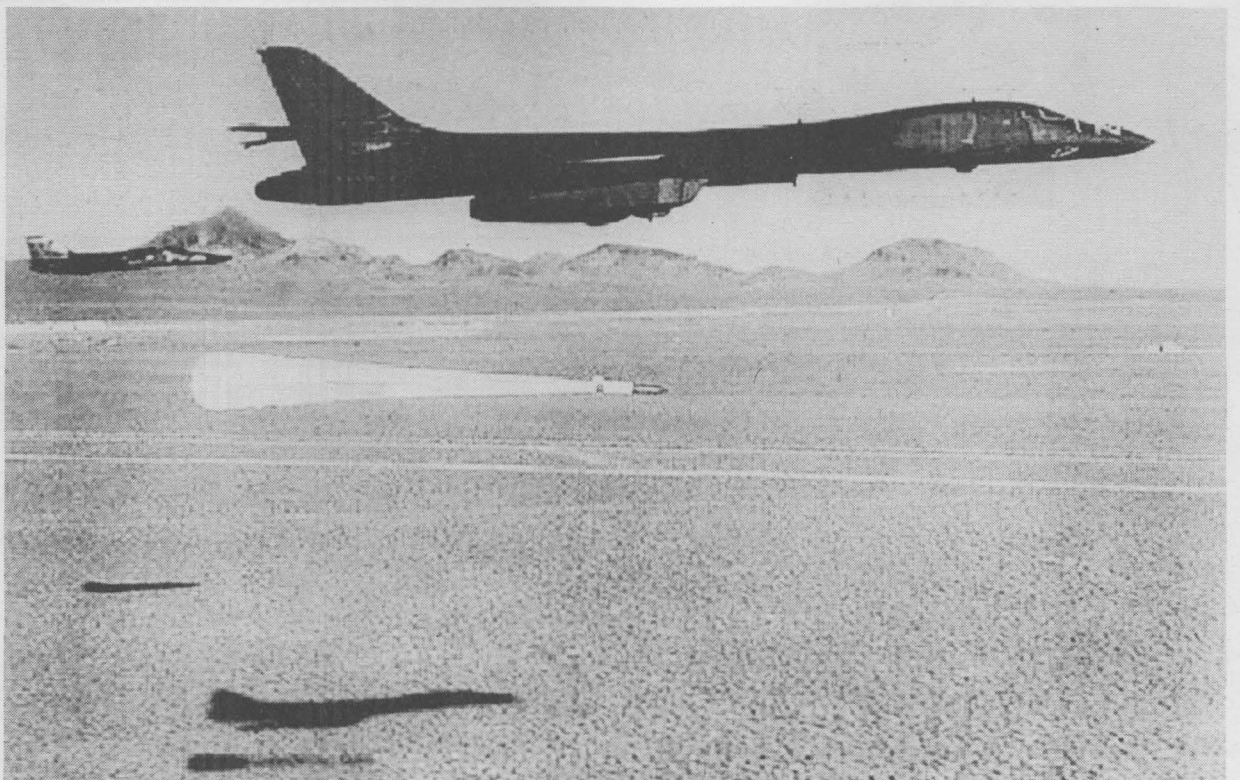
LAYING IT DOWN — A B1-B bomber on a test run deploying the B61-11 at the Tonopah Test Range. Sandia conducted 13 full-scale drop tests this year, three in Alaska and 10 at the Tonopah facility.
